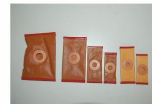
*Manufacturing various types of membranes which are used in the different pneumatic systems*
